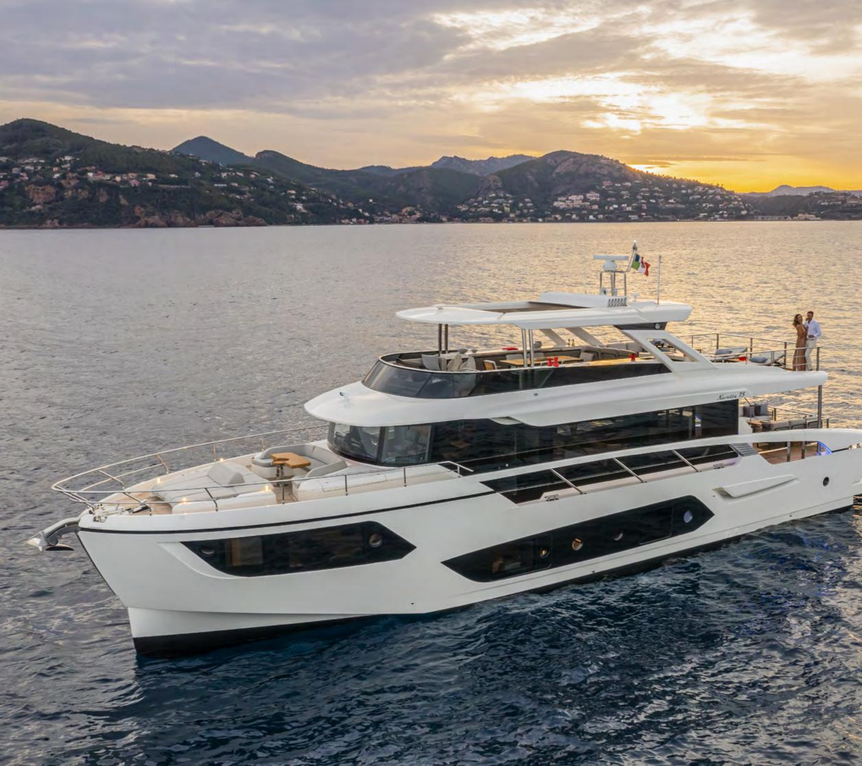
Doing this study, however, I also realize that, when travelling at 10 knots, wonder within a miracle, consumption is just six litres per mile, which would basically be 65 litres per hour: basically, the consumption of a RIB with two latest-generation outboards. Incredible. Accelerating, consumption certainly rises, but it always remains in a very low range, an irrefutable sign of a particularly well-designed hull.
