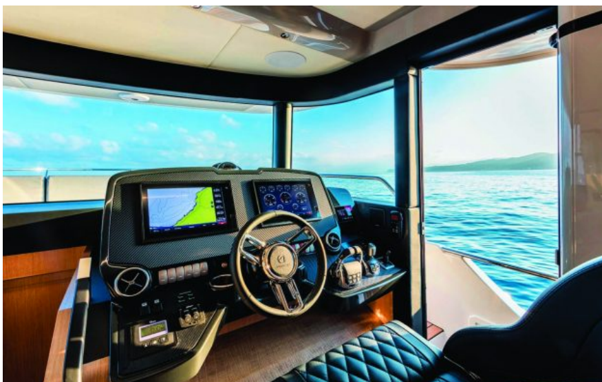
The vertical, one-piece screen means there are very few blind spots from the lower helm
